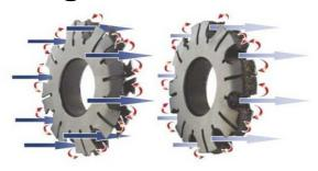
The filtration technology developed by Magnom removes sub-micron and larger-sized contaminants from hydraulic fluid using a combination of magnets and specially formed steel plates to collect particles. Housed around central magnets, the steel plates transmit magnetic fields that attract ferrous and other magnetically sensitive particles into collection zones between the plates.
